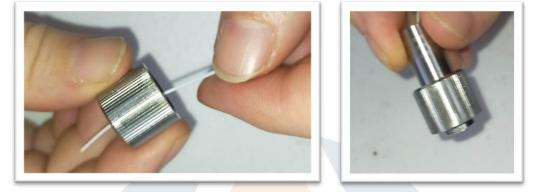
Pass the Wetlink body through the fiber and screw to the connector. Make sure the oring is present and greased.
