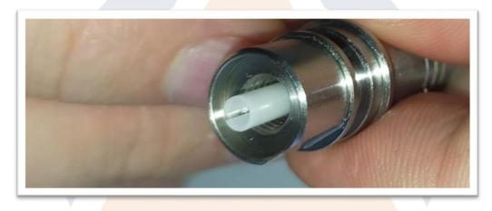
Insert the ferrule guide inside the connector and screw all the way down with the provided tool.
