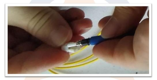
Pull the fibre from the yellow outer sheath.
