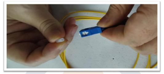
Using side cutters break off the blue shell
