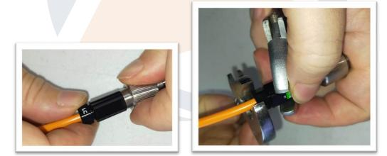
The fibre connector is now fully assembled and ready to be spliced to your ROV tether. Don't forget to put the o-ring!
