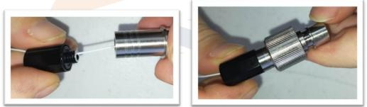
Insert the Wetlink gland and packing nut on the water-resistant sheath and fish the fibre through it.
