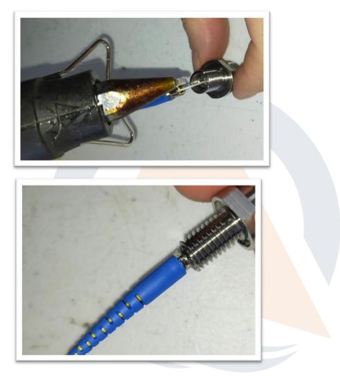
The fibre bulkhead is now fully assembled and ready to be spliced to a connector of your choice.
