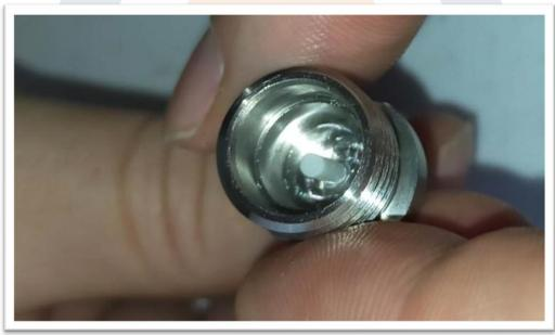
Fish the packing screw on the fibre and insert in the back of the bulkhead.
