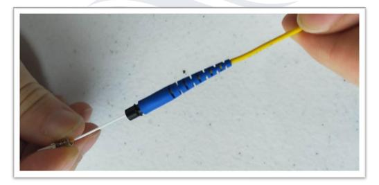
Your fibre is now ready to be inserted into the bulkhead or connector.
