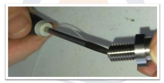
Retrieve the left-over outer sheath and pass the fibre through it. This will act as a bend stiffener and protect your fibre.
