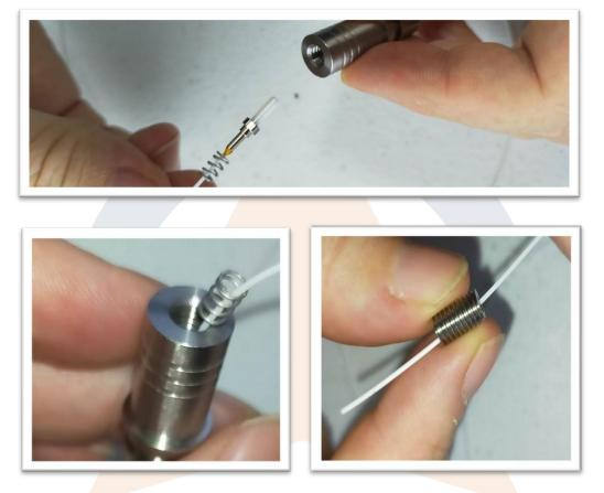
Insert the packing screw into the back of the connector using a flat screwdriver. Turn the connector, not the screwdriver. Be careful as this step can damage the fibre.
