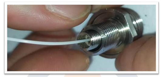
Insert the packing screw into the back of the bulkhead using a flat screwdriver. Turn the bulkhead, not the screwdriver. Be careful as this step can damage the fibre.
