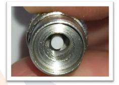
Insert the ceramic ferrule inside the connector.
