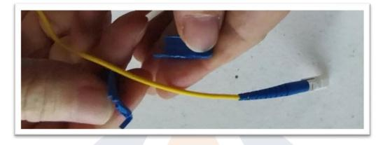
Remove the white clip using side cutters.
